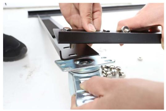
2. Start with a corner caster. Align the holes of the long-side bar, short-side bar and a caster (with a brake). (See the figure above)
